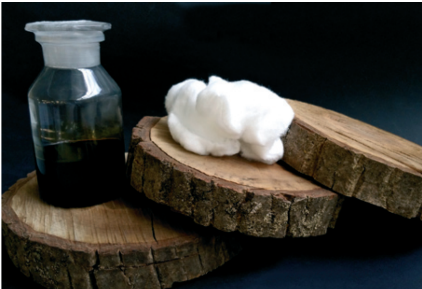
A bonding agent for thermoset plastic is made from waste material from the pulp industry.
